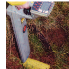
Unique signal traced using Receiver
